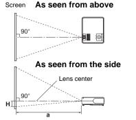
a is the distance (m) between the lens and the screen, and corresponds to a range of 1.45 m to 11.29 m. H is the height from the image bottom to the center of the lens.
